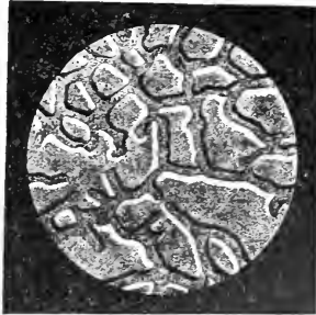
FIG. 4.—Copper containing 0.5 per cent. of antimony. Slowly cooled. Magnified 56 diameters. Viewed by oblique light.
